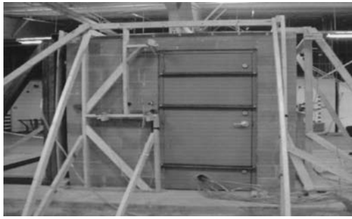
Fig. 9. Full-scale CMU specimen with instrument frame
